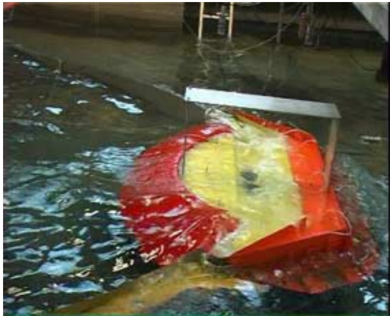
Overtopping on the Wave Dragon scale 1:50
