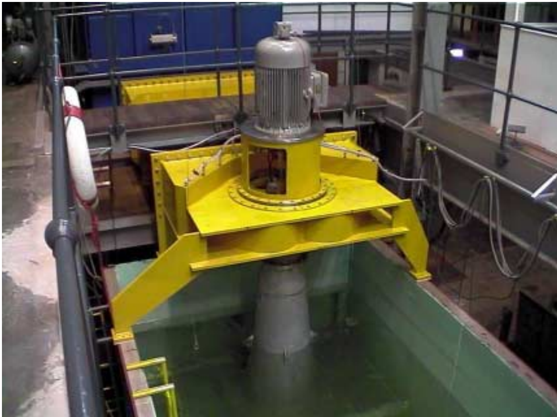
The tested Wave Dragon-model at the turbine at test stand. Same turbine to be applied in scale 1:4.5 project.
